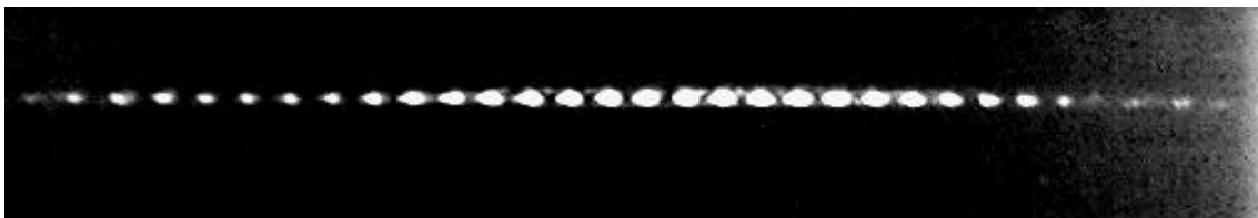
Figure 8-b : Outputs of a star coupler device made with the organic-inorganic material.
